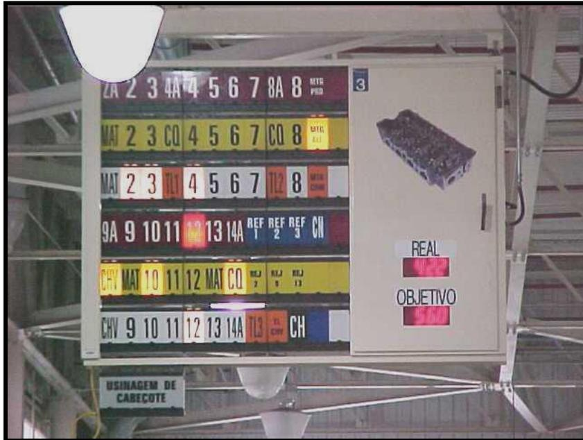
*Fig. 1: A typical andon board*
